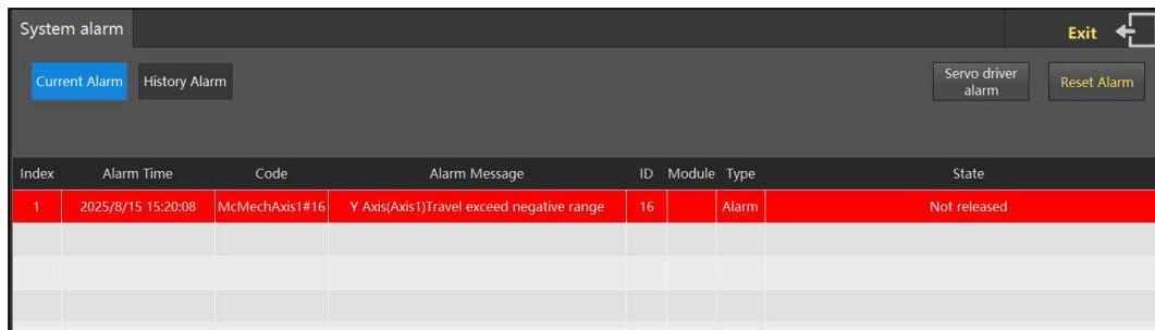
Figure 7-15 Debug - alarm log
